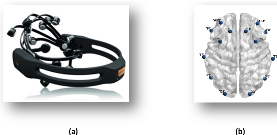
Figure 2. (a) Emotiv EPOC headset; (b) position of EEG electrodes on the human scalp.
